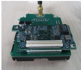
Fig. 6. The sensor board MTS300CA connected to the NESCTM
