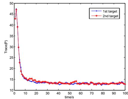
Fig. 6. The average trace of error covariance in the first scenario of two-target tracking
