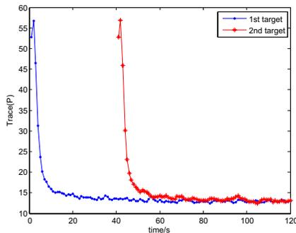
Fig. 9. The average trace of error covariance in the second scenario of two-target tracking
