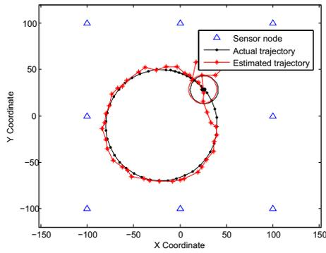
Fig. 2. The trajectory of single-target tracking
