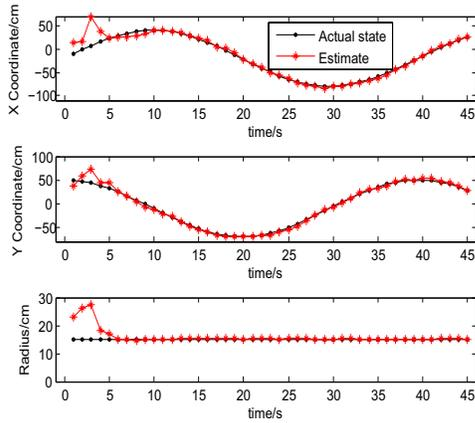
Fig. 3. The comparison of the estimate and true state of single-target tracking
